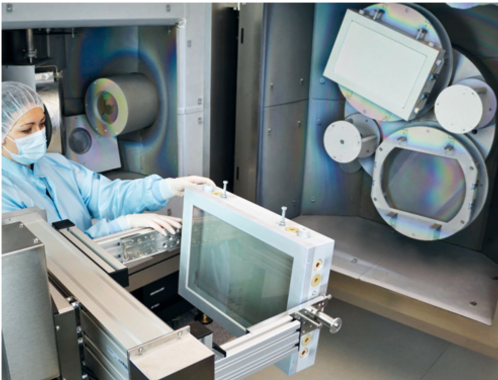
"Teresa", the largest IBS machine, suitable for substrates up to Ø 550 mm
