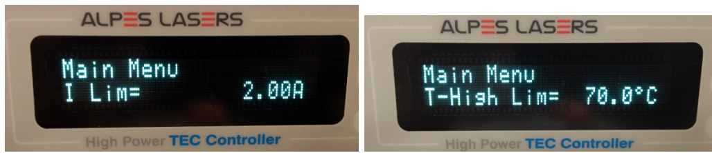
Figure 6.5.: TC-3 temperature controller GUI I Lim and T High Lim .
