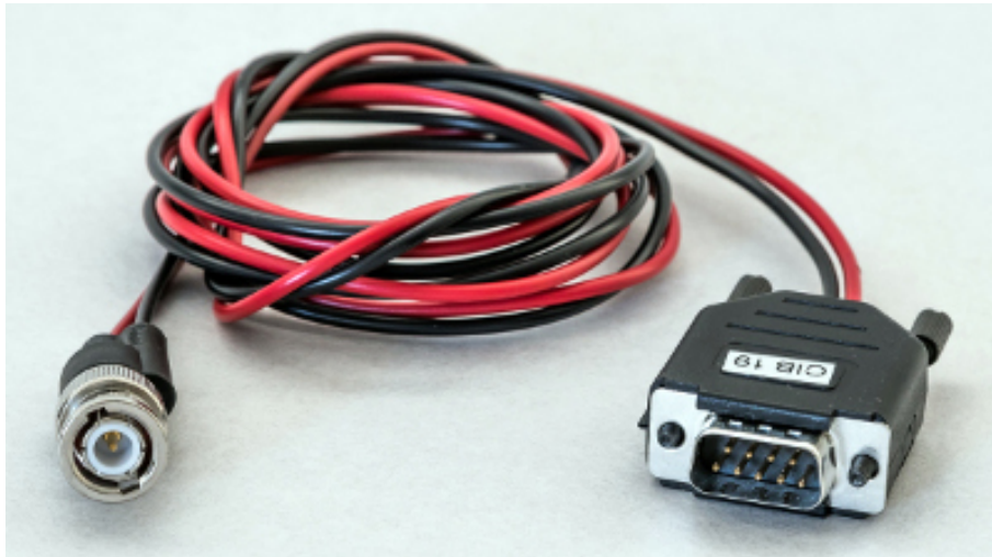
Figure 5.11.: C-LDX-HHL cable connecting the HHL housing to the LDX-3232 driver.
