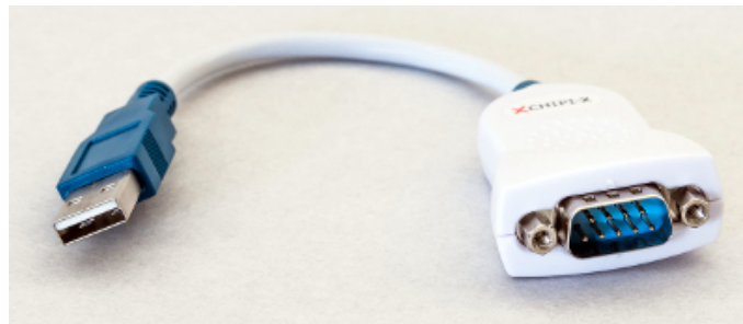
Figure 3.1.: USB-RS232 adapter cable.
