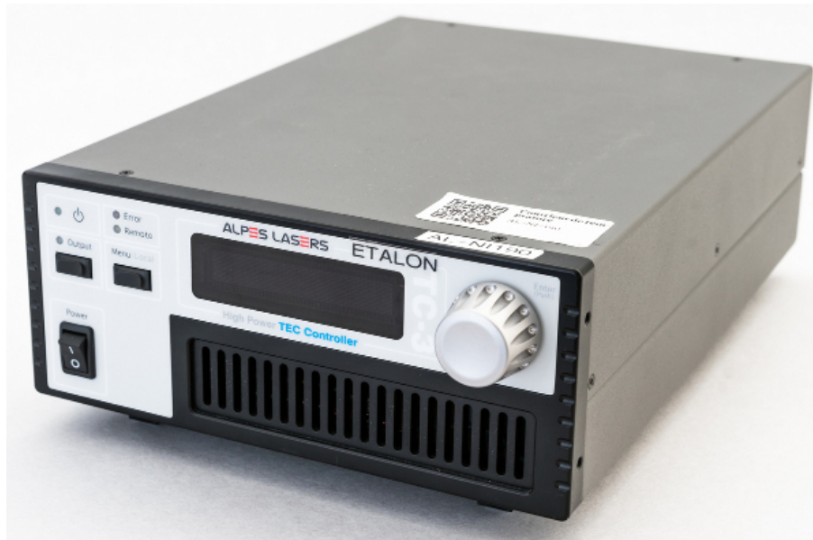
Figure 6.2.: TC-3 temperature controller.
