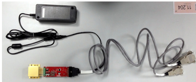
Figure 5.8.: HHL housing connected directly to the S-2 pulser, itself connected to the C-S-2-TC3 cable, with the the S-2 pulser power supply.
