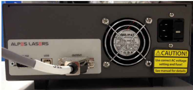
Figure 6.3.: TC-3 temperature controller back panel.
